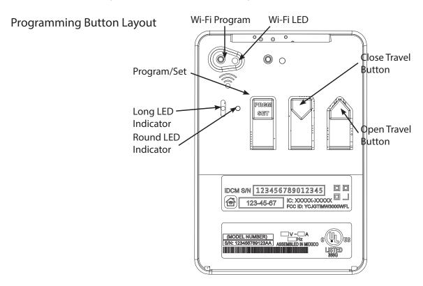
**NOTE**: Each programming step has a 30 second time limit for completion after the function is initiated. After 30 seconds, both LED's will illuminate RED indicating time has expired and the step must be restarted. Restart the step as many times as necessary to complete the programming.
